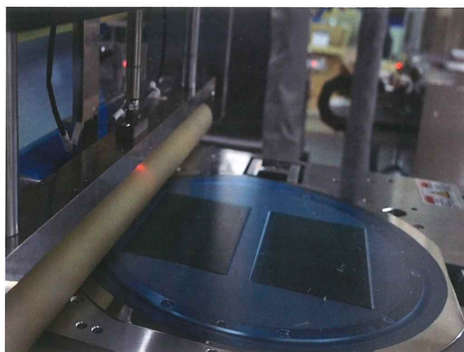
貼膜區 Tapping Station
